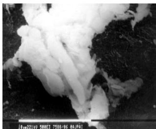
Fig. 1 Scanning Electron Micrograph of matrix surface containing 27.7% BA
